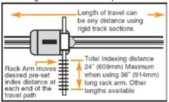
automatically stops and reverses direction while at the same time indexing the gun/torch. It can be programmed to weld or not weld during indexing. Carriage is predrilled for quick mounting of the indexing unit (sold separately).
